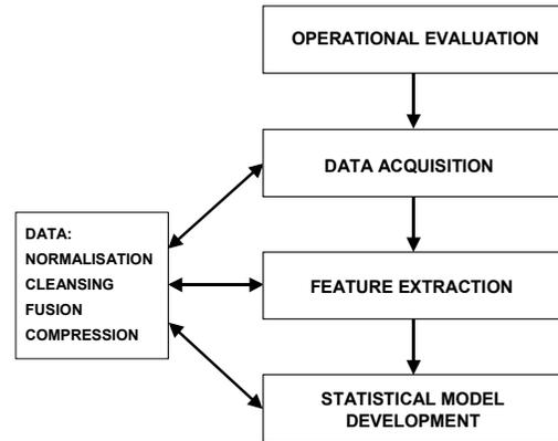
Fig. 2. Flow chart showing the principle data operations for the implementation of a health monitoring system [2].
