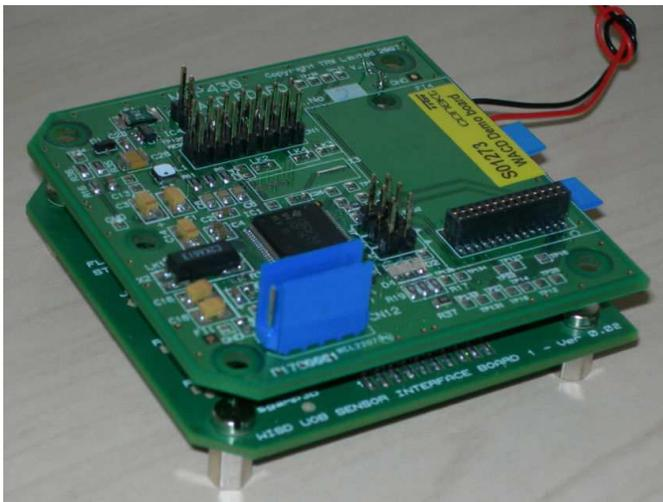
Fig 11 Two boards make up the sensing module for the flight trail system. The lower board is a low power strain gauge interface and the upper board carries the MSP430 processor. The RF board is removed in this photo.
