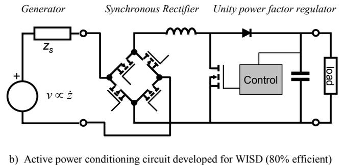
Fig 9 Comparison of a typical passive power conditioning used for energy harvesting with the active system used in the WISD project to improve efficiency of the energy conversion process.
