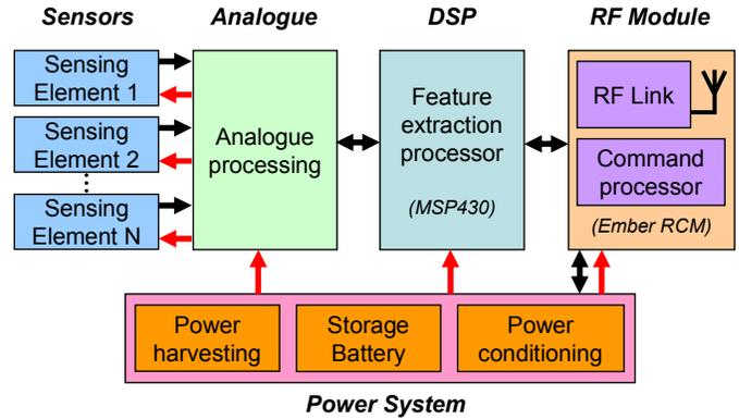
Fig. 5. Architecture of the remote wireless sensing node, showing the main sub-systems of the device.
