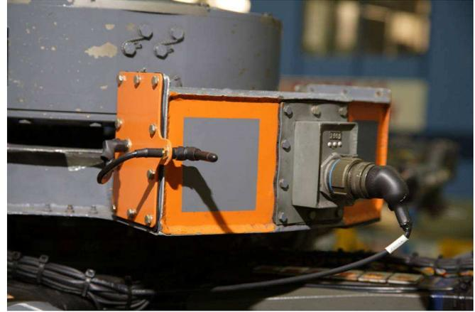
Fig 12 The sensor module is fitted within an enclosure mounted on the rotor hub. The aerial of the WISD system can be seen.
