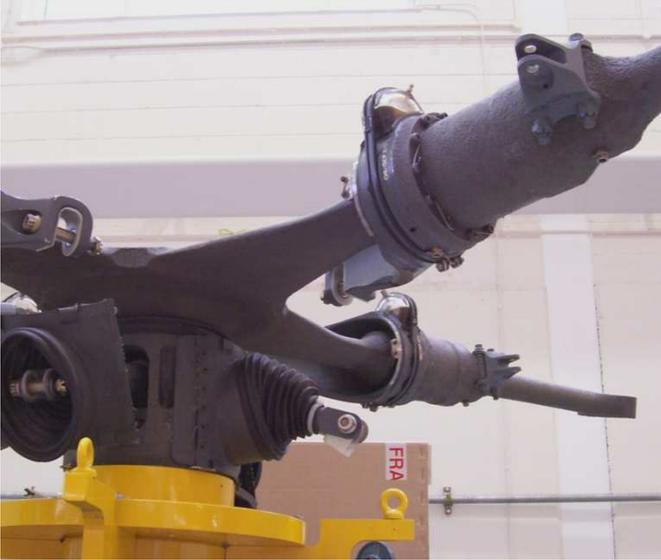
Fig. 3. Main rotor hub of a Lynx helicopter, made up of flexible and jointed components. The WISD project sought to measure the cumulative bending stress experienced by the flexible centre cruciform.
