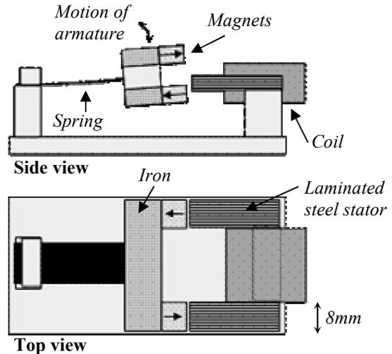
Fig. 7. Diagram of the harvester developed for the WISD project featuring nonlinear compliance response and high magnetic loading.
