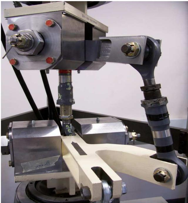
Fig. 4. The pitch link, shown here as a pair undergoing laboratory wear testing to gather data for developing feature extraction algorithms. The link has a ball joint at each end which the WISD project aimed to monitor.
