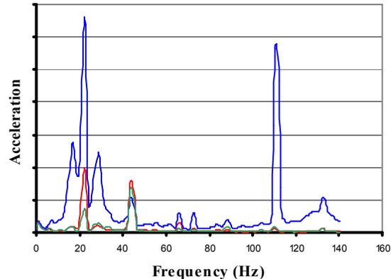
Fig. 6. Measured vibration spectrum at several helicopter body locations during forward flight. The amplitude data is omitted for commercial reasons, however vibration peaks of >1g can be found in some locations.
