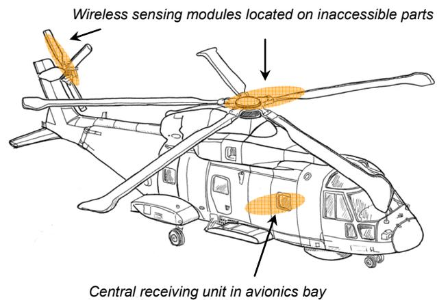
Fig. 1. Sketch showing how safety critical parts of a rotorcraft structure could be monitored with a wireless sensing system, particularly when the components to be monitored are in difficult to reach locations such as the rotor head.
